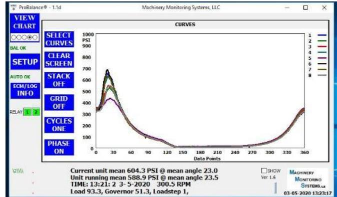
The screens above shows the phased and un-phased cylinder pressure plots. Combustion statistics that are tracked (and can be alarmed on) include:
