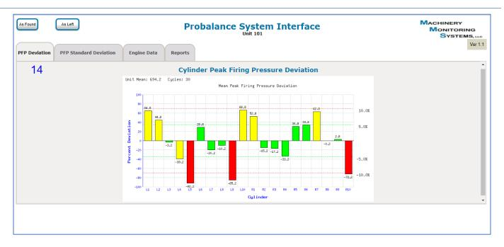
The screen above shows the web page which is wirelessly available in the engine room for display on a tablet computer or smartphone with just a Web Browser. This screen allows the operator to view the engine balance live while making adjustments to each cylinder's fuel valve.
