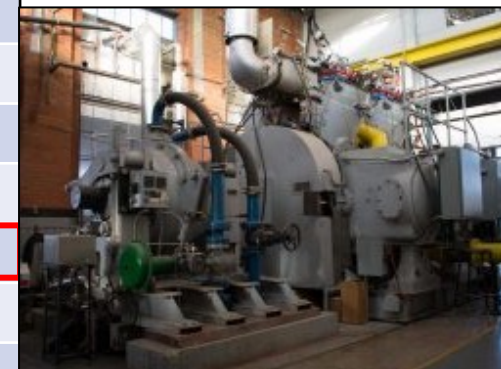
CSU Energy Institute GMV-4 Cooper Bessemer Test Engine
