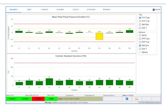
The screen above shows the web page which is wirelessly available in the engine room for display on a tablet computer or smartphone with just a Web Browser. This screen allows the operator to view the engine balance live while making adjustments to each cylinder's fuel valve.
